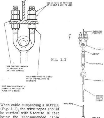
when cable suspending a ROTEX (Fig. 1.1), the wire ropes should be vertical with 5 feet to 10 feet being the recommended cable length. It is suggested that turn-buckles be used at the upper ends of the cables to make leveling easier. In all cases, suitable cable clamps and thimbles or swaged fittings should be used to attach the cables. (Fig. 1.2)
