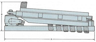
Drawings are representative of ROTEX models to show principal dimensions only. Complete dimensional drawings of individual models, showing location of foundation bolts and other details, are available on request.
