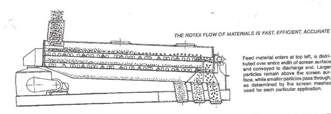
Feed material enters at top left, is distributed over entire width of screen surface and conveyed to discharge end. Larger particles remain above the screen surface, while smaller particles pass through, as determined by the screen meshes used for each particular application.
