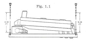
To cable suspend the ROTEX, four wire rope assemblies are required, one attached to each corner. These cables should be of improved plow steel quality or equivalent. The recommended cable size for each model series is shown in the following table.
